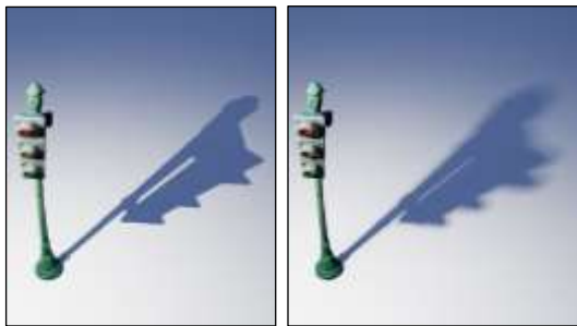
Figure 3 – Shadows using a traditional shadow map (left), and distance fields (right) (Epic Games, 2021).
